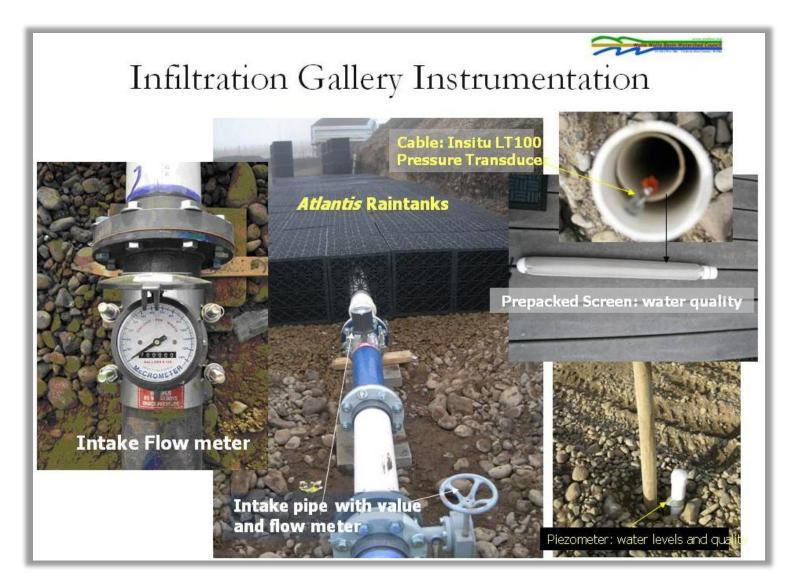
Figure 61. Infiltration Gallery monitoring equipment (2009)
