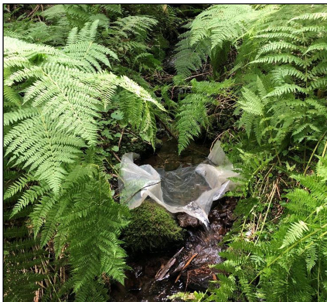
Figure 6. Field teams used plastic sheeting to channel spring water for a volumetric flow measurement.
