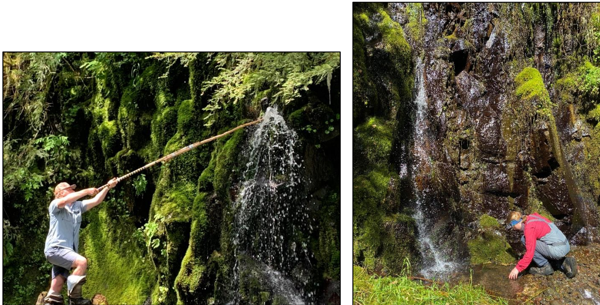
Figure 15. Left: WWBWC staff collect water from a gushet spring. Right: Staff place water quality sensors directly into a spring-fed pond to measure water temperature, conductivity, pH, and dissolved oxygen.
