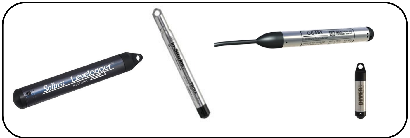
Figure 4. Pressure transducers used in the Shallow Aquifer Monitoring Network. Continuously monitored wells were equipped with one of the above types of pressure transducers.
