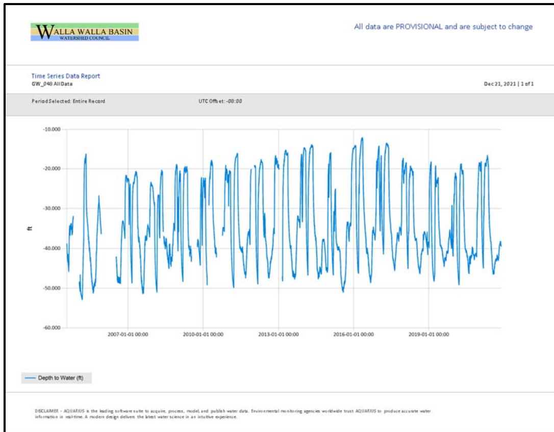
Figure 23. Pressure transducer data (blue line) in feet below ground surface for the well GW_048 located in the WWBWC's Shallow Aquifer Monitoring Network.
