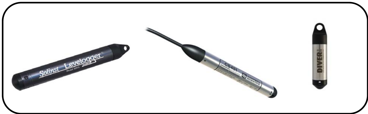
Figure 4. Pressure transducers used in the Shallow Aquifer Monitoring Network. Continuously monitored wells were equipped with one of the above types of pressure transducers.
