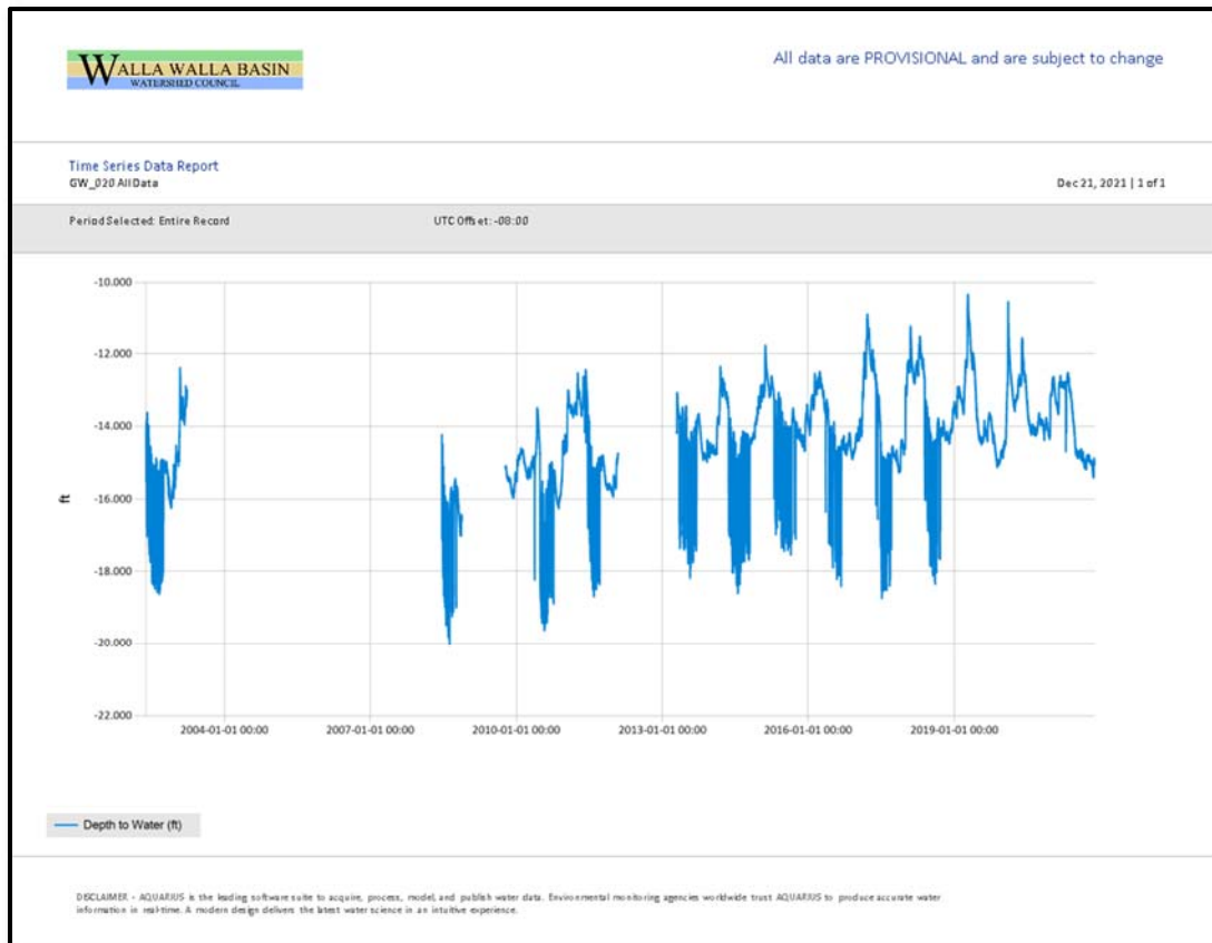
Figure 28. Pressure transducer data (blue line) in feet below ground surface for the well GW_020 located in the WWBWC's Shallow Aquifer Monitoring Network.
