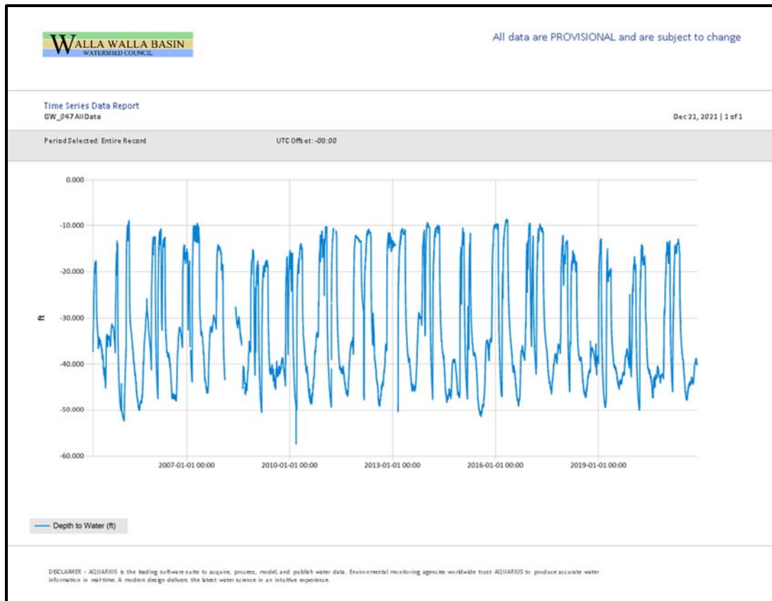
Figure 22. Pressure transducer data (blue line) in feet below ground surface for the well GW_047 located in the WWBWC's Shallow Aquifer Monitoring Network.
