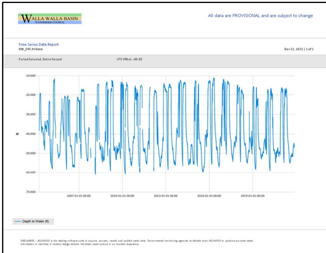
Figure 20. Pressure transducer data (blue line) in feet below ground surface for the well GW_045 located in the WWBWC's Shallow Aquifer Monitoring Network.
