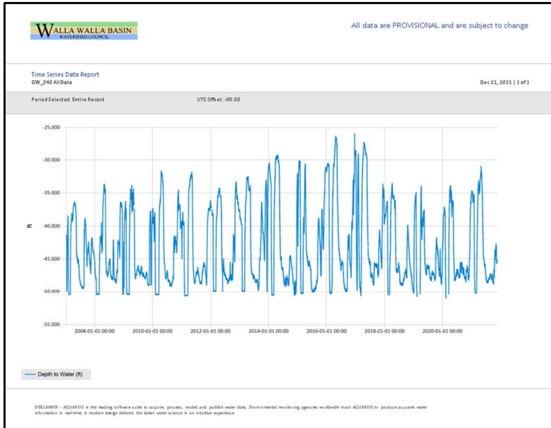
Figure 19. Pressure transducer data (blue line) in feet below ground surface for the well GW_040 located in the WWBWC's Shallow Aquifer Monitoring Network.
