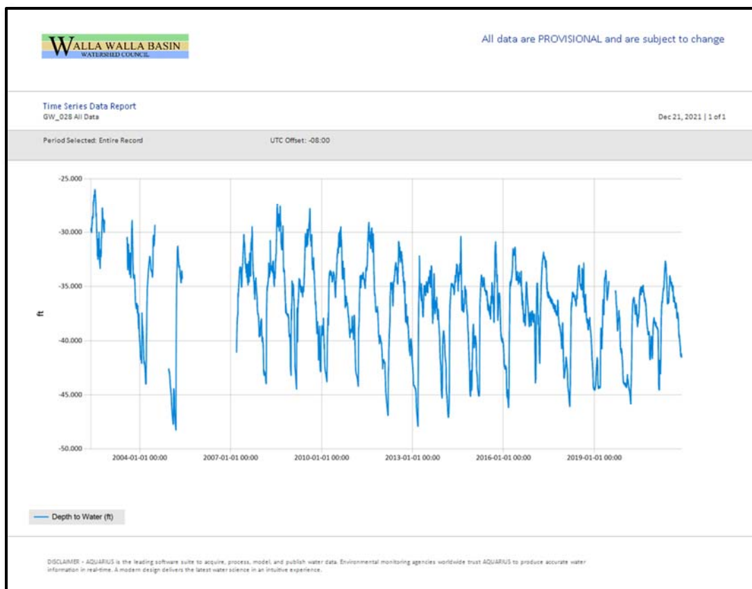
Figure 12. Pressure transducer data (blue line) in feet below ground surface for the well GW_28 located in the WWBWC's Shallow Aquifer Monitoring Network.
