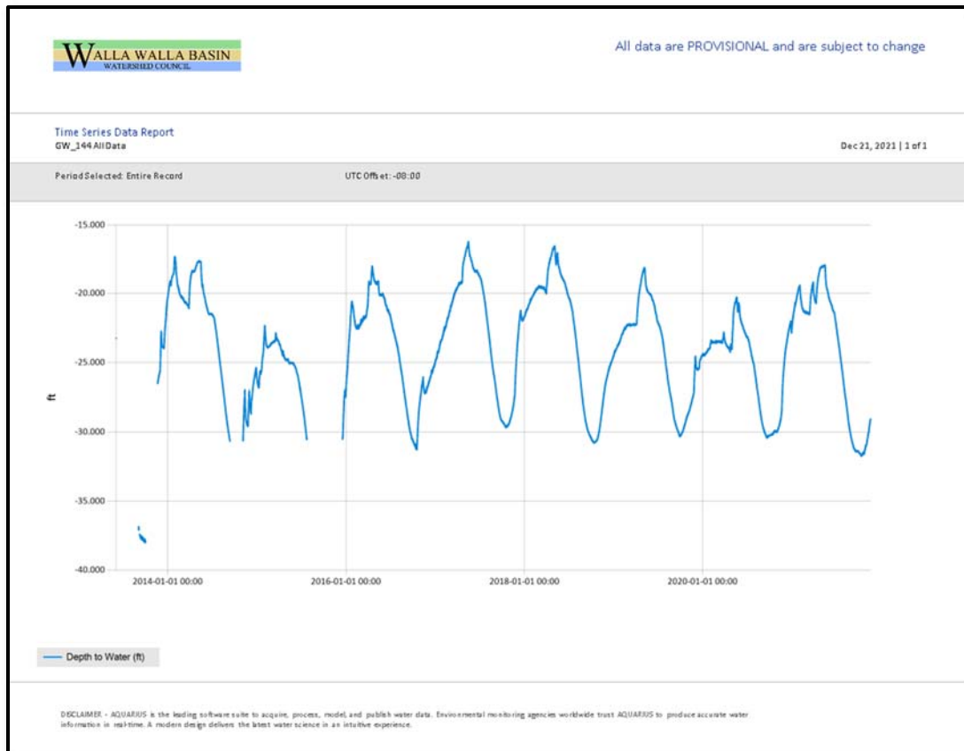
Figure 26. Pressure transducer data (blue line) in feet below ground surface for the well GW_144 located in the WWBWC's Shallow Aquifer Monitoring Network.
