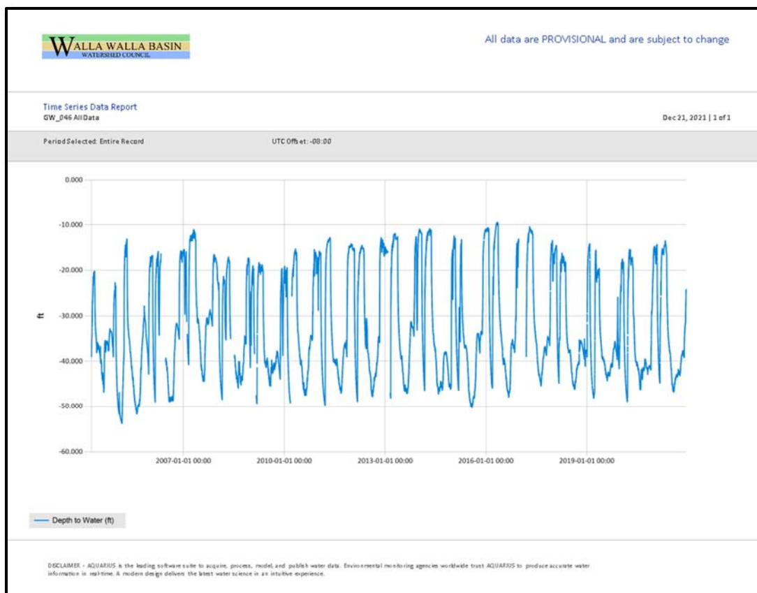
Figure 21. Pressure transducer data (blue line) in feet below ground surface for the well GW_046 located in the WWBWC's Shallow Aquifer Monitoring Network.
