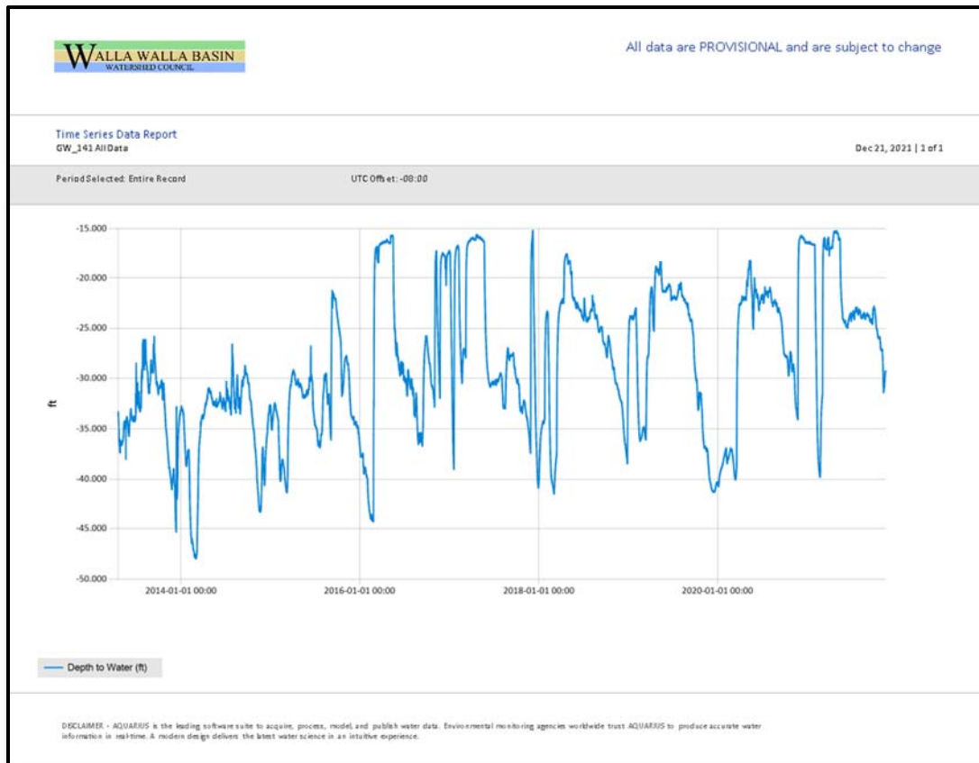
Figure 18. Pressure transducer data (blue line) in feet below ground surface for the well GW_141 located in the WWBWC's Shallow Aquifer Monitoring Network.
