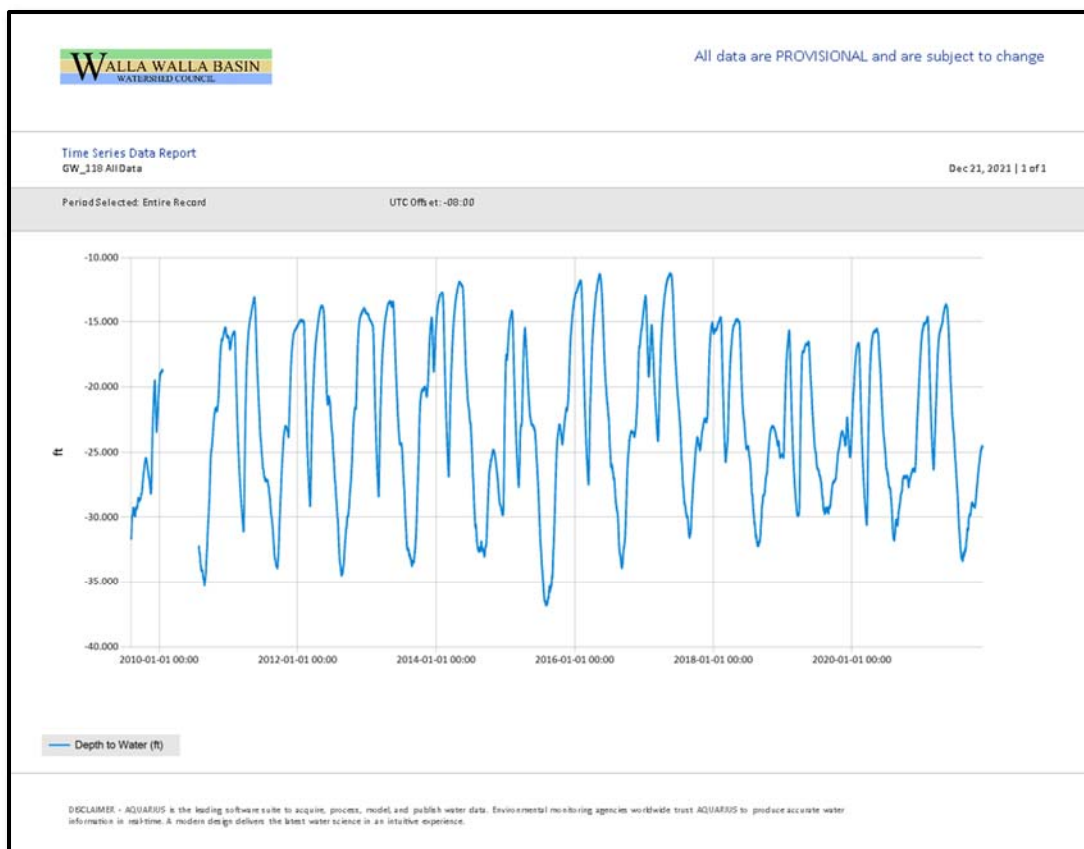
Figure 24. Pressure transducer data (blue line) in feet below ground surface for the well GW_118 located in the WWBWC's Shallow Aquifer Monitoring Network.
