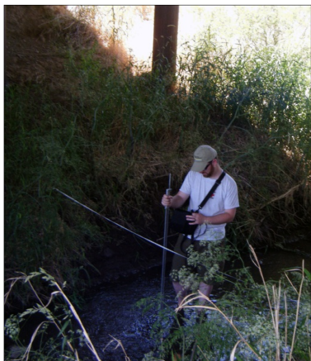
WWBWC personnel conducting a discharge measurement
