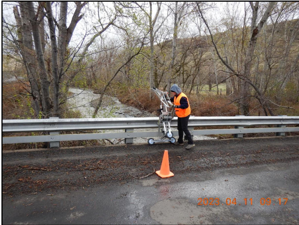
Figure 5. Staff setting up a bridge board flow measurement on North Fork Walla Walla River (S-104) using a Price AA current meter and AquaCalc Pro Plus.
