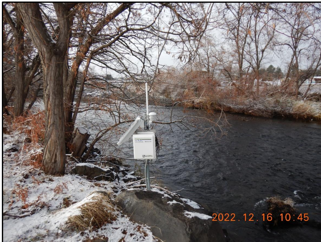
Figure 4. At this near real-time monitoring site on the South Fork Walla Walla River (S-107), a cabled sensor secured to a boulder collects water level data. A communication cable transmits the information to a data logger and radio housed in the gauge box. Using radio telemetry, water level, and temperature data are sent to the WWBWC office to be processed and published online.
