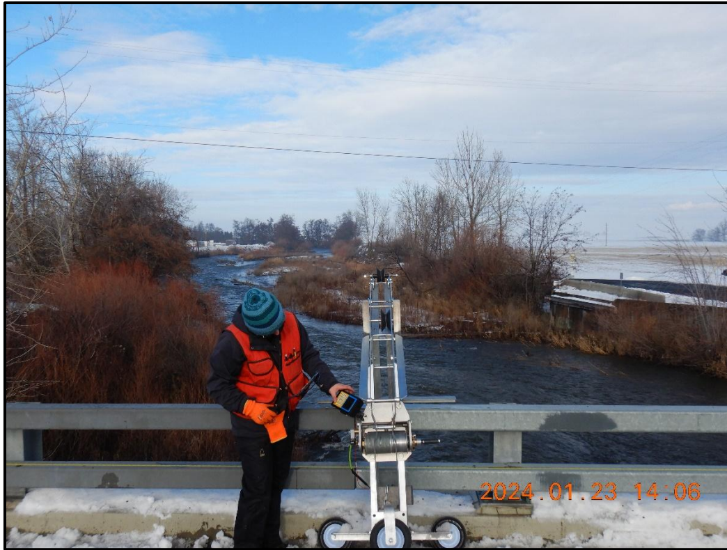
Figure 6. Staff performing a high flow bridge measurement on Walla Walla River at Tum-A-Lum Bridge (S-107) using a Price AA current meter and AquaCalc Pro Plus.
