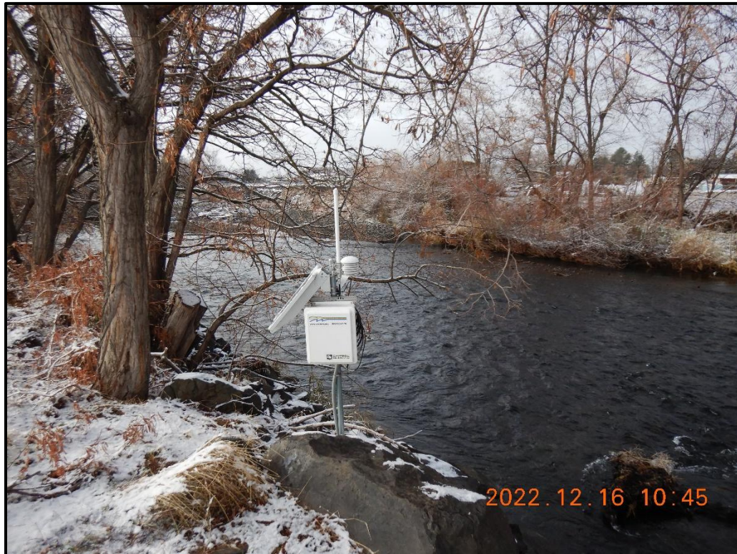
Figure 5. At this near real-time monitoring site on the South Fork Walla Walla River (S-107), a cabled sensor secured to a boulder collects water level data. A communication cable transmits the information to a data logger and radio housed in the gauge box. Using radio telemetry, water level, and temperature data are sent to the WWBWC office to be processed and published online.
