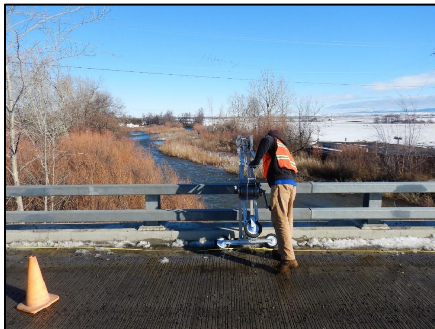
Figure 5. Staff performing a high flow bridge measurement on Walla Walla River at Tum-A-Lum Bridge (S-107) using a Price AA current meter and AquaCalc Pro Plus.
