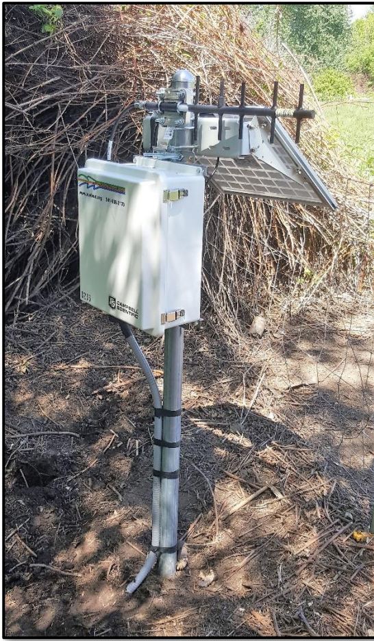
Figure 4. At this near real-time monitoring site on the East Little Walla Walla River, a cabled sensor secured to a T-post and staff gauge in the channel collects water level data. A communication cable transmits the information to a data logger and radio housed on the streambank. Using radio telemetry, water level and temperature data are sent to the WWBWC office to be processed and published online.
