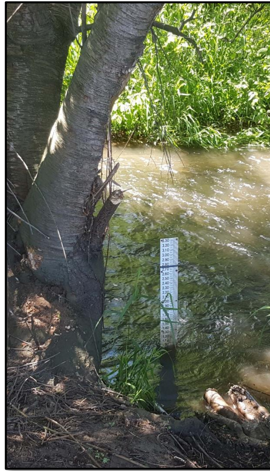
Figure 4. At this near real-time monitoring site on the East Little Walla Walla River, a cabled sensor secured to a T-post and staff gauge in the channel collects water level data. A communication cable transmits the information to a data logger and radio housed on the streambank. Using radio telemetry, water level and temperature data are sent to the WWBWC office to be processed and published online.
