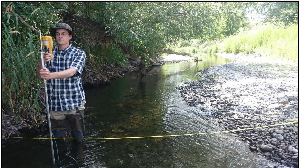
Figure 5. Staff taking a wading flow measurement on Mill Creek using a FlowTracker2 acoustic Doppler velocimeter.
