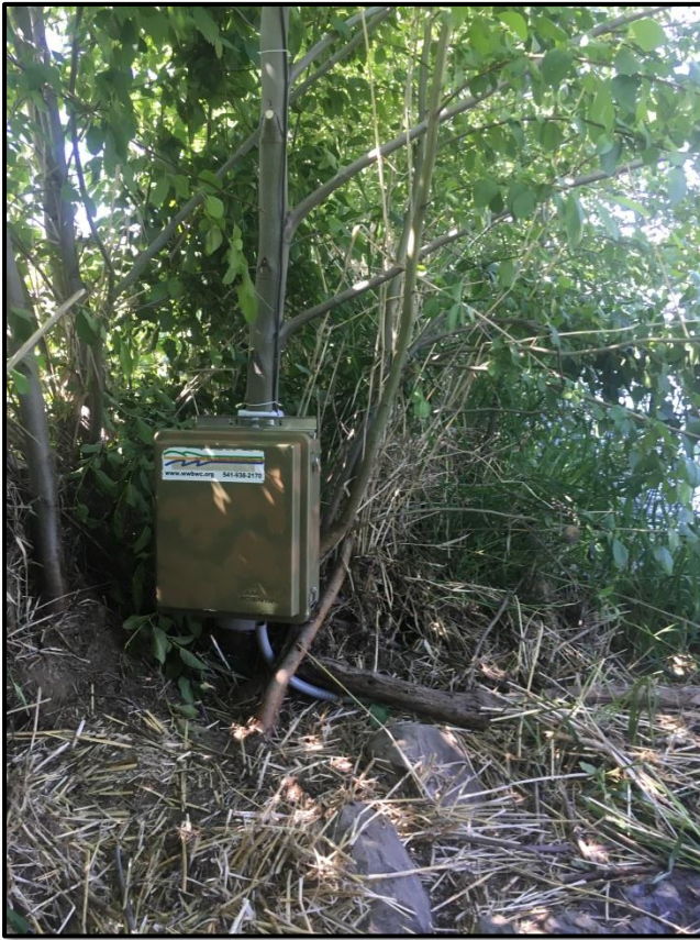
Figure 4. At this near real-time monitoring site on the Walla Walla River (S-106), a cabled sensor secured to a T-post and staff gauge in the channel collects water level data. A communication cable transmits the information to a data logger and radio housed on the streambank. Using radio telemetry, water level and temperature data are sent to the WWBWC office to be processed and published online.
