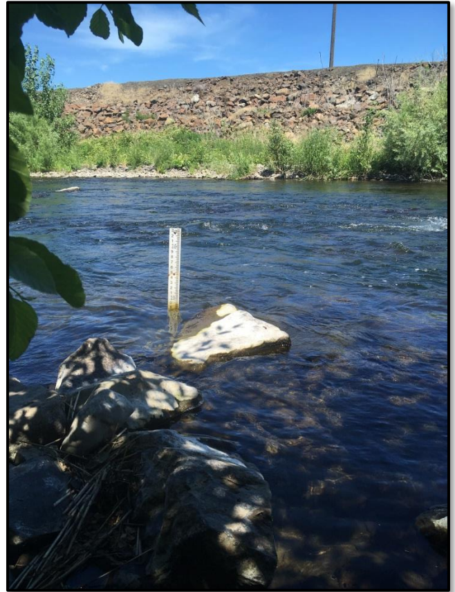
Figure 4. At this near real-time monitoring site on the Walla Walla River (S-106), a cabled sensor secured to a T-post and staff gauge in the channel collects water level data. A communication cable transmits the information to a data logger and radio housed on the streambank. Using radio telemetry, water level and temperature data are sent to the WWBWC office to be processed and published online.
