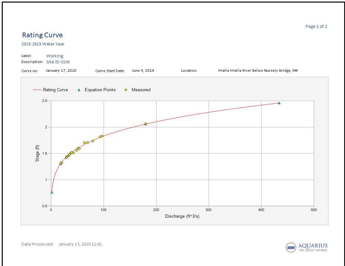
Figure 7. Rating Curve for the Walla Walla River below Nursery Bridge. Yellow dots represent manual discharge measurements. Blue triangles show rating points.
