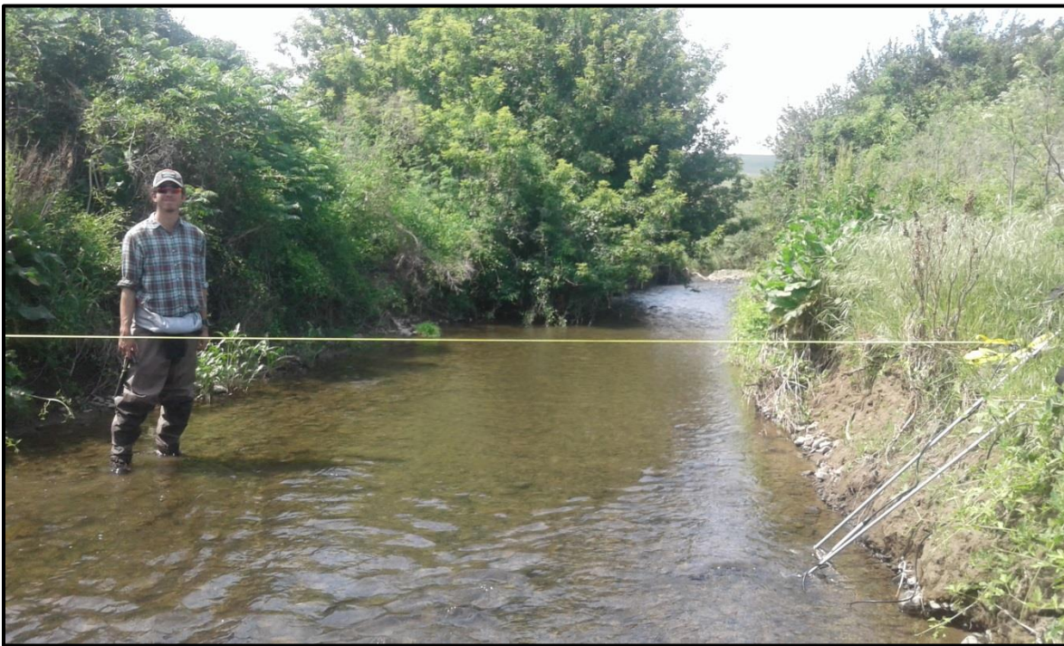
Figure 5. Staff setting up a flow measurement on Pine Creek (S-416T) using a FlowTracker2 acoustic Doppler velocimeter.
