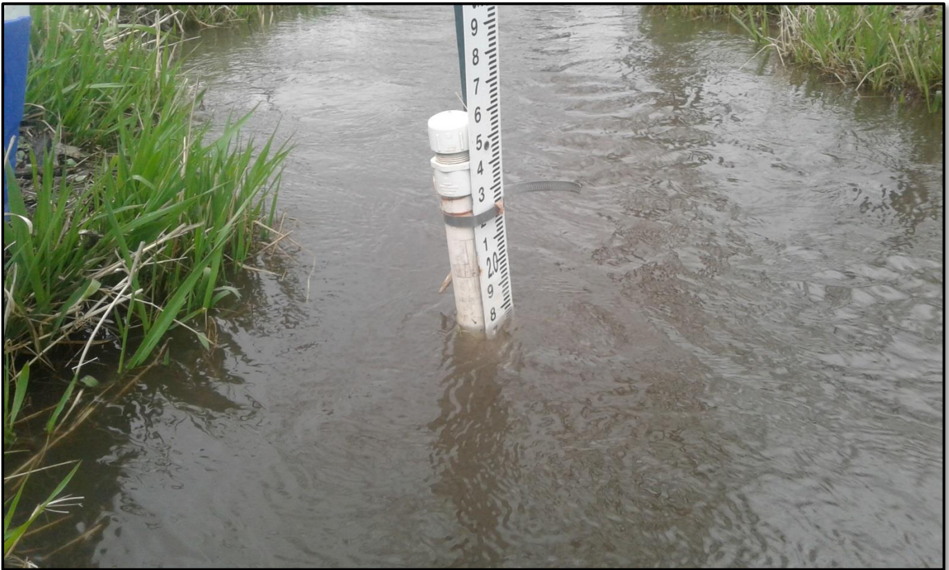
Figure 6. At this stand-alone monitoring site on the West Little Walla Walla River (S-222), a staff gauge and perforated PVC stilling well with a suspended pressure transducer. Typical equipment installed at stand-alone monitoring sites that were visited quarterly for manual data download
