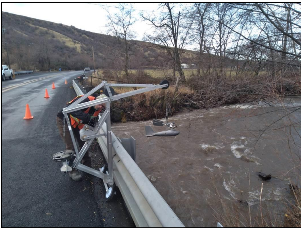
Figure 5. Staff setting up a bridge board flow measurement on South Fork Walla Walla River (S-103) using a Price AA current meter and AquaCalc Pro Plus.
