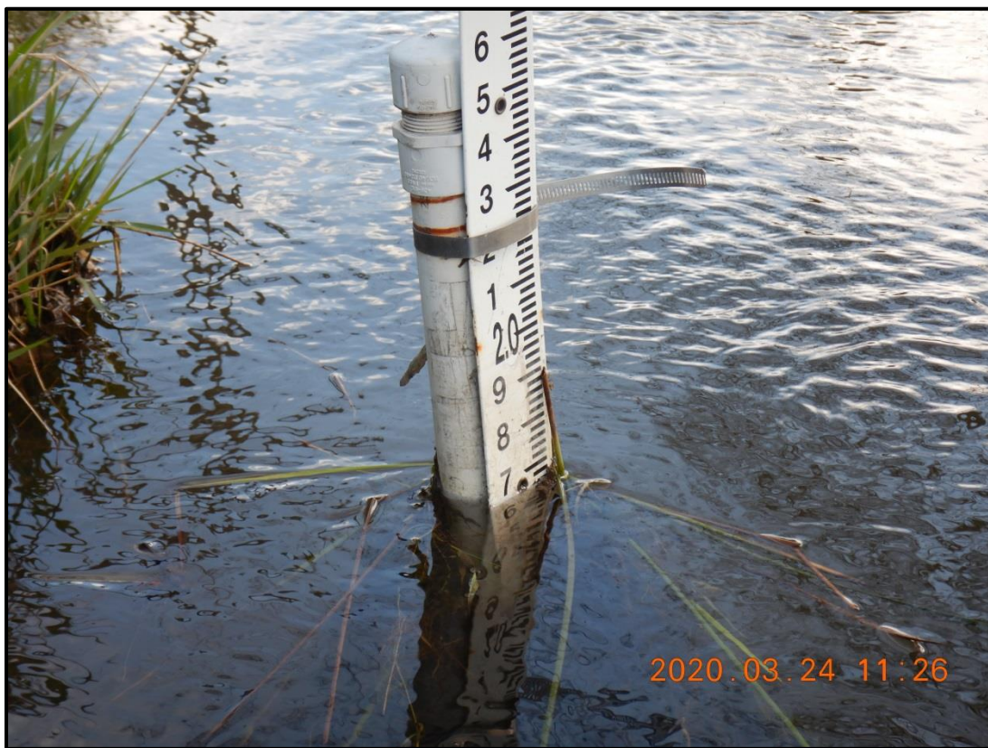
Figure 6. At this stand-alone monitoring site on the West Little Walla Walla River (S-222), a staff gauge and perforated PVC stilling well enclose a suspended pressure transducer. These are the typical components installed at stand-alone monitoring sites that were visited quarterly for manual data download
