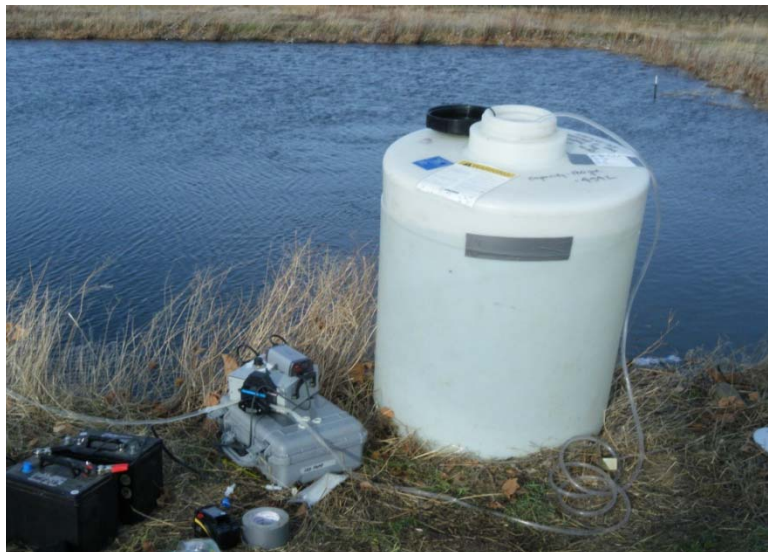
Figure 4.2 Tracer injections at Hudson Bay aquifer recharge project. 400-liter container pumped at 950ml/min using a peristaltic pump.
