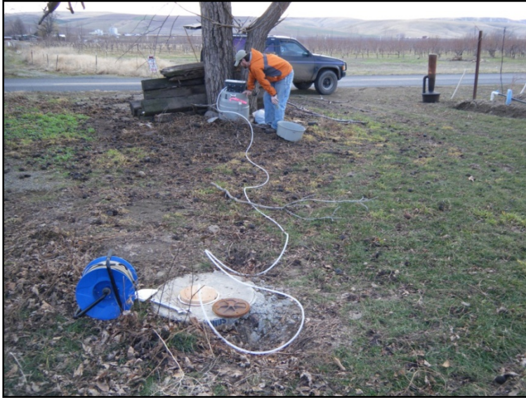
Figure 4.3 Automatic sampler setup at observation well Gw_118.
