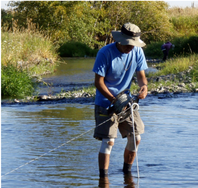
5.2. Photograph of Arístides Petrides deploying the cable in the Walla Walla River, having just passed the cable through a “pig-tail” support post.
