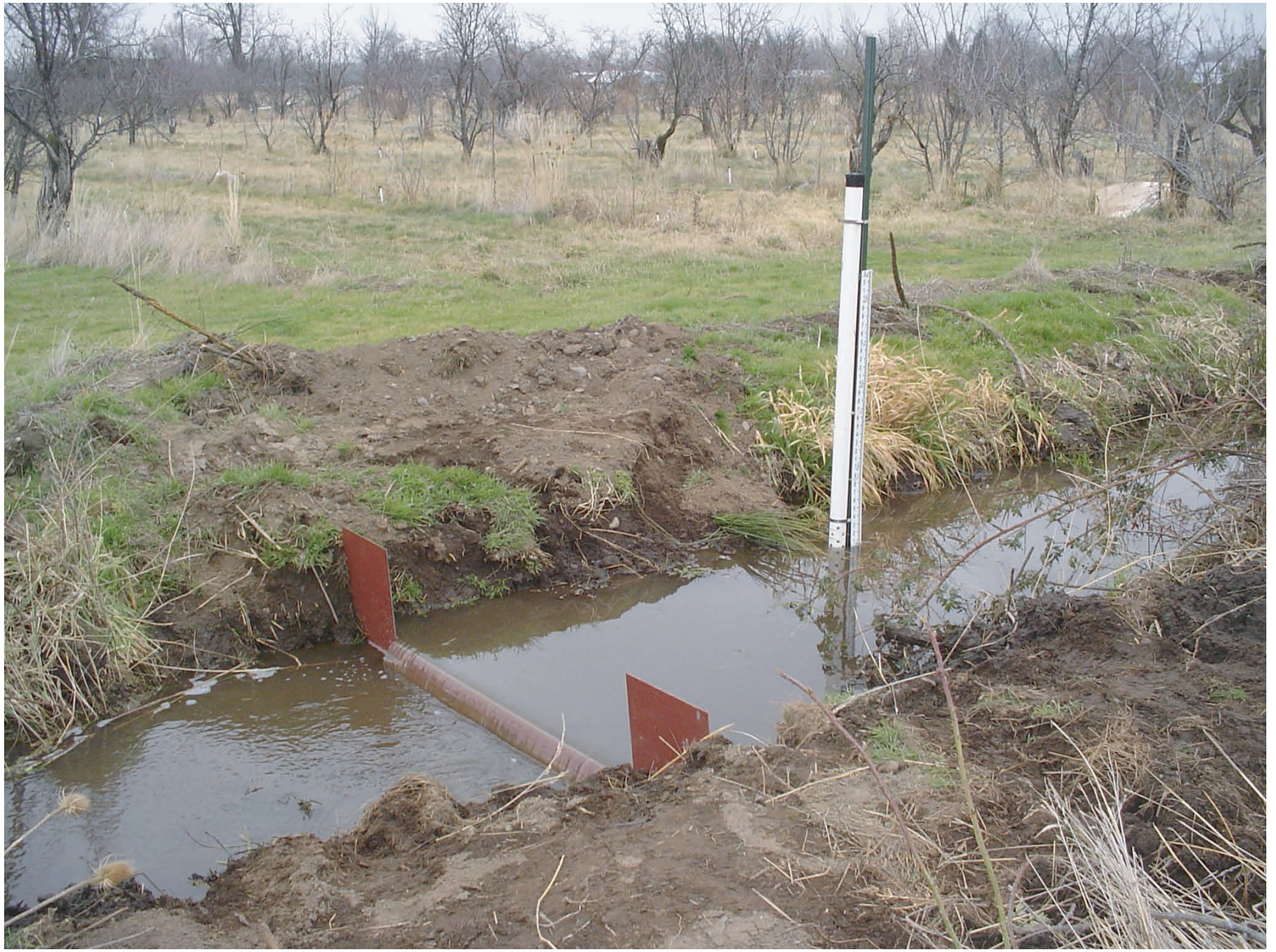
Figure 16. Photograph of the measurement weir on the branch ditch leading onto the Test Site.
