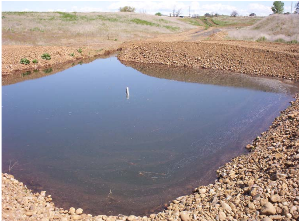
Figure 14. The lower basin late in the test. Tube in middle of basin contains digital transducer and an attached staff gauge. Upper basin is at base of slope in upper part of photo.
