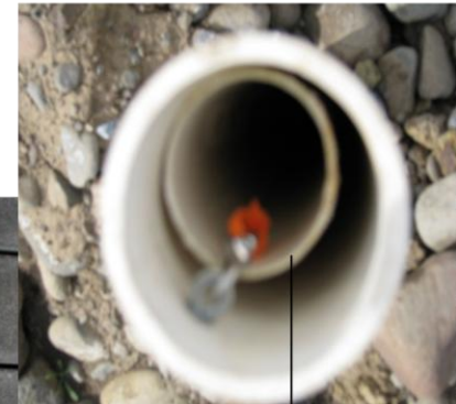
Cable: Insitu LT100 Pressure Transducer
