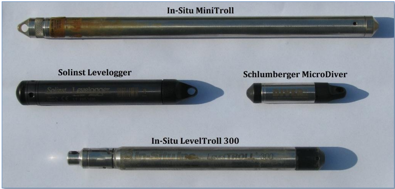
Figure 4. Pressure transducers used in the Shallow Aquifer Monitoring Network. Continuous wells have one of these pressure transducers deployed.
