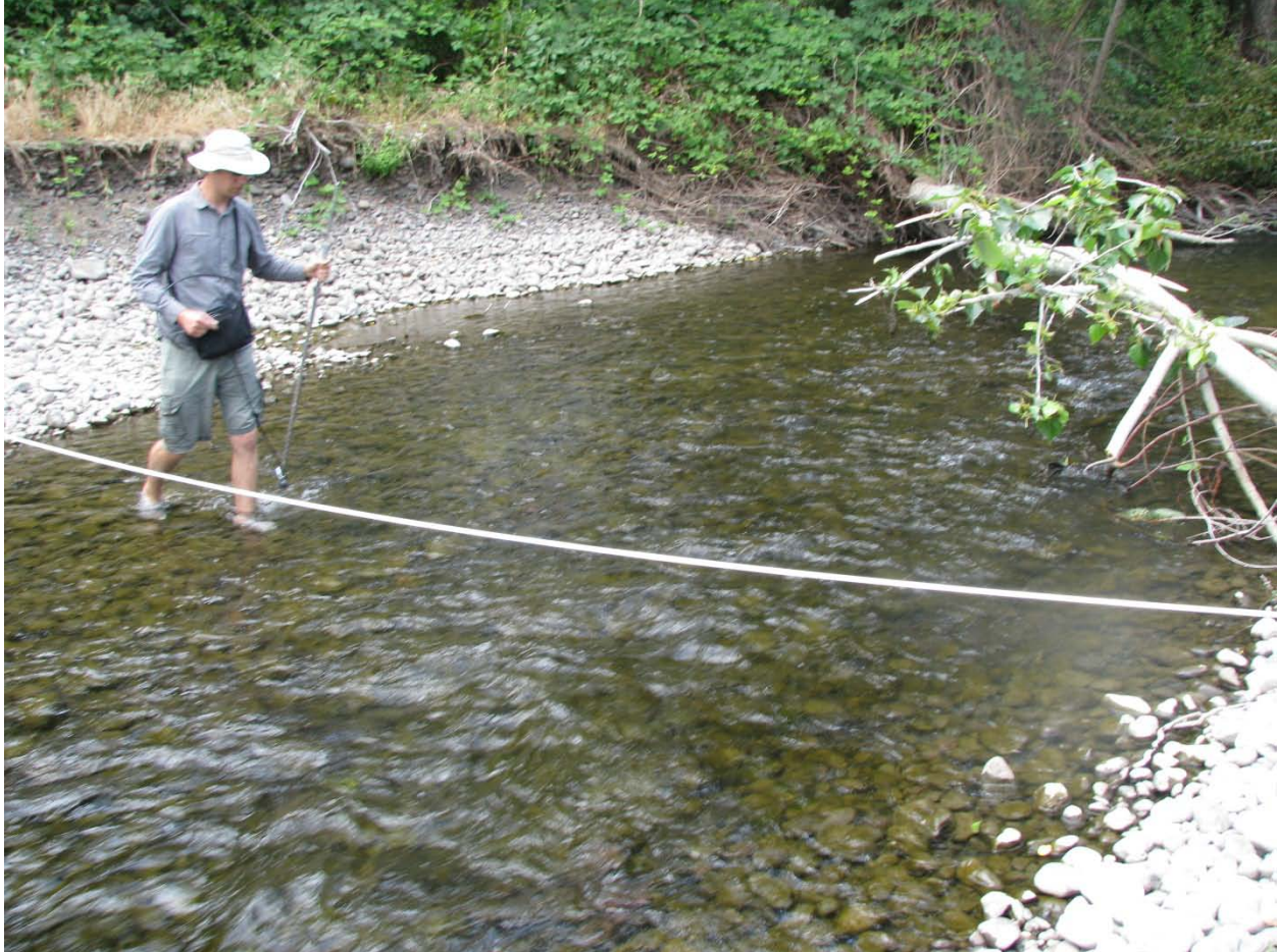
Figure 6. Instantaneous flow measurement of the Walla Walla River: A tape is hung across the river. At points along the tape, depth and velocity values are recorded. Discharge of a cell = Depth * velocity * cell width. This is how flow is estimated for instantaneous flow measurements.
