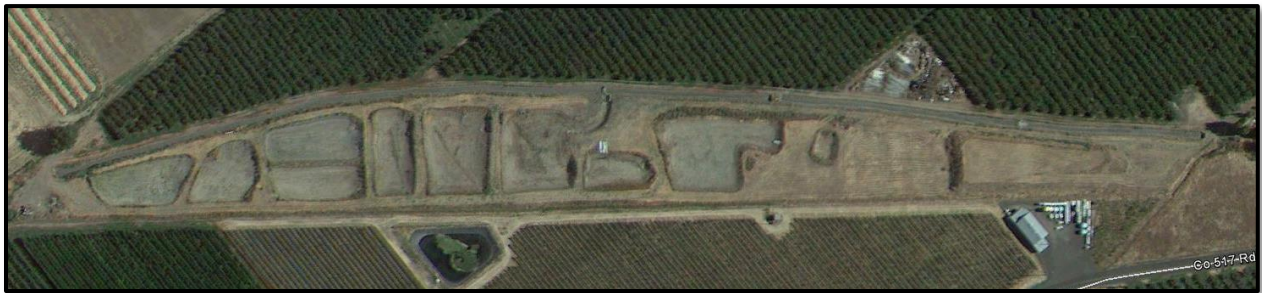
Figure 11 - Aerial photo of the Johnson site from 2013 showing the current configuration of the site with 10 spreading basins and 3 active infiltration galleries (between the spreading basins and the pile of fill).
